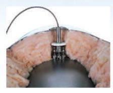
The high temperature HT-R probe is 2.25 inches in diameter and magnetically attachable to the steel surface. It can be applied to any steel surface greater than 8 inches in diameter and
