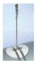
The all temperature stationary AT-S probe is 6 inches in diameter. It has been designed for semi-permanent installation at a site and is attached to a steel surface using banding. The AT-S probe is ideally attached at a site that requires frequent monitoring, ensuring consistent measurements time and again. These probes can be fixed to any steel surface greater than 8 inches in diameter and at temperatures up to 500°C, 930°F.
