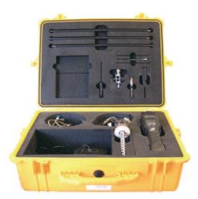
The Hydrosteel Complete Kit includes both the low temperature and high temperature probes, giving you everything you need to begin monitoring active corrosion. The Kit also includes a one year Gold Replacement Service\* giving you total piece of mind that you will always have an instrument available for measurements.
