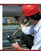
Totally non-intrusive, Hydrosteel 6000 is the first flux monitor to measure active corrosion in steel pipes and vessels in petrochemical service at temperatures up to 500 °C, 930 °F.
