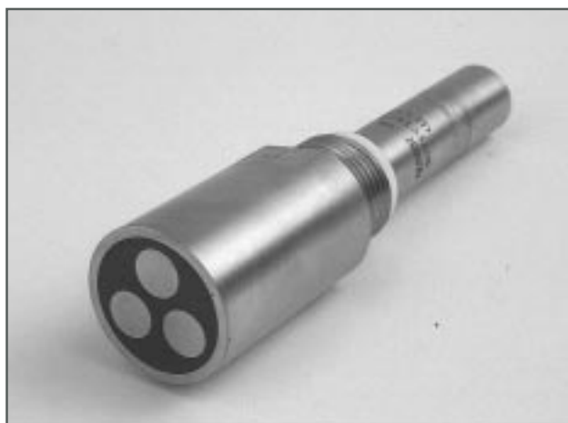
A flush 3 electrode LPR probe in AC mounting style.
