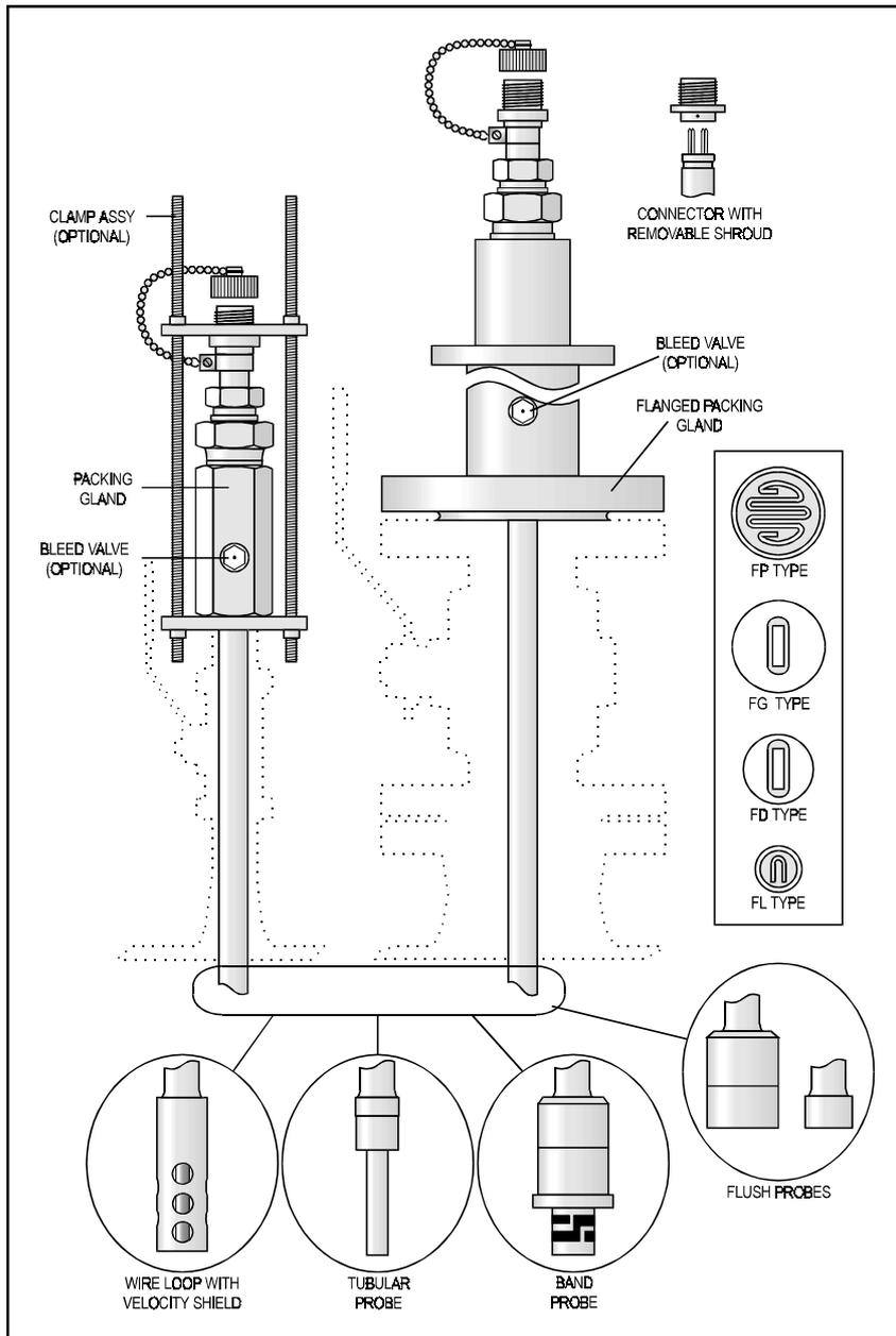
A comprehensive range of ER probes for making metal loss measurements in processes up to 1000 psi and 260°C with options up to 1500 psi, and 450°C.
