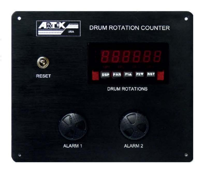
Operationally, the Artex Drum Rotation Counter numerically counts drum revolutions while movingdown the well bore, then reverses the numerical count while traveling out of the well bore. This numeric count increases one number per revolution of the wireline drum in both directions.
