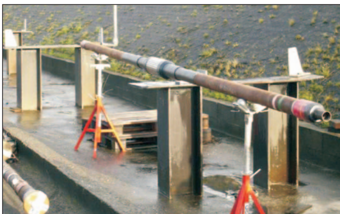
Fig. 11 Test run assembly; "PetroCeram Sleeve" positioned in the middle
