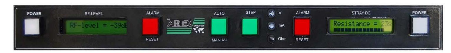
The RF & stray voltage monitor supervises 4 parameters: induced voltage, current, ground resistance and RF level. RF is monitored continuously, the others parameters are monitored sequentially or can be user set to one of the three. In case of an excess level, an audible and visible alarm is generated. Besides that, an alarm relay trips and can be connected to external circuitry as a safeguard.
