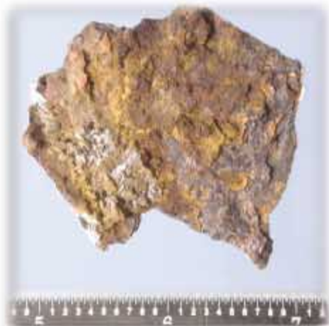
Example of General Corrosion
