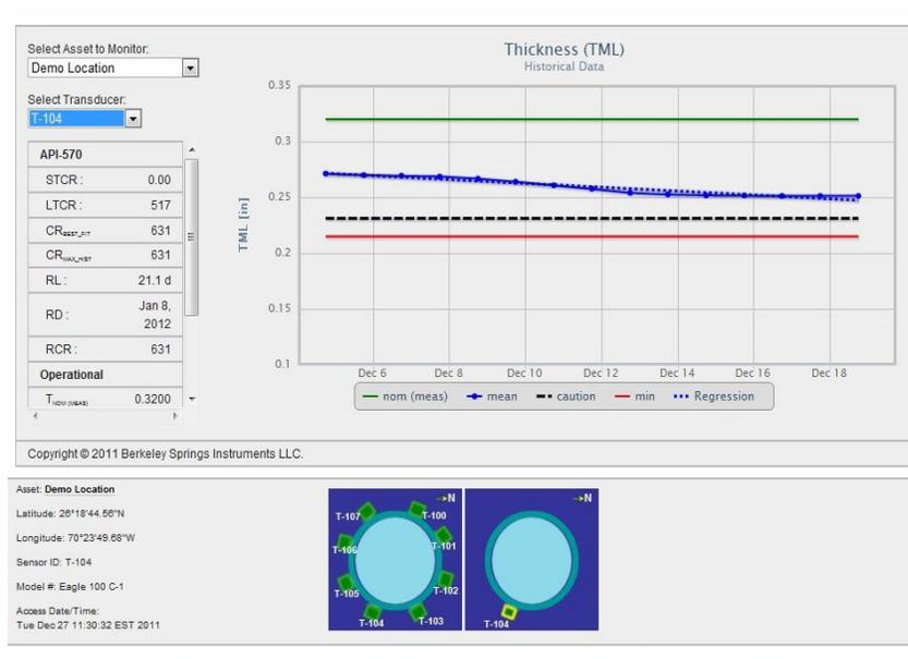
Figure 4. User interface providing real-time mechanical integrity information to the user and updated API-570 calculations regarding remaining useful life and retirement dates. End view of current pipe data under review is shown.
