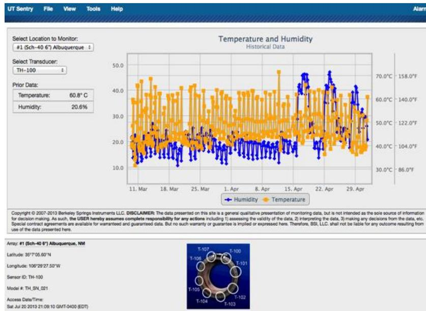
Figure 7. Temperature/humidity data monitoring user interface. Temperature and humidity information are time-stamped to associate each event with the UT data and corrosion rates.
