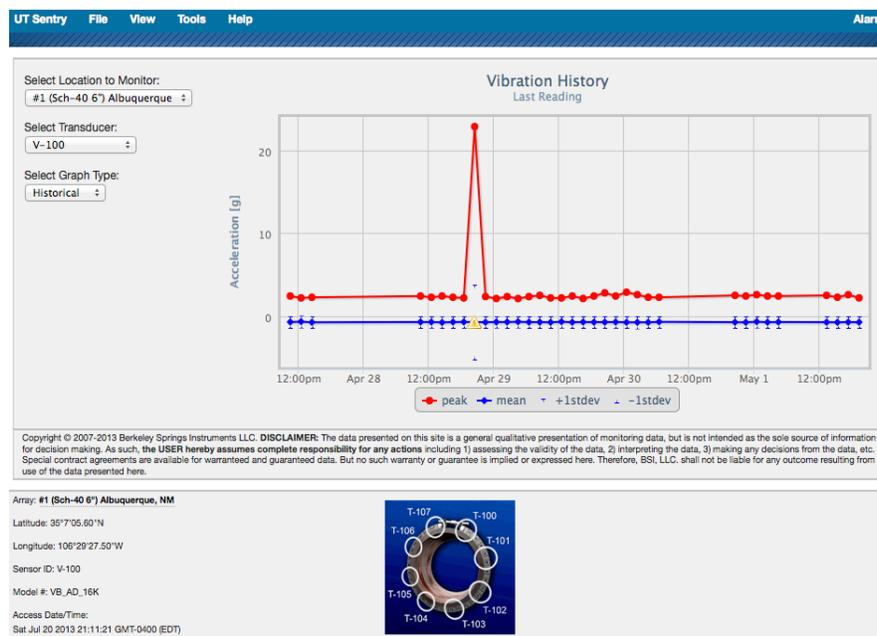
Figure 6. Vibration data monitoring user interface. Vibration information is time-stamped to associate each event with the UT data and corrosion rates.
