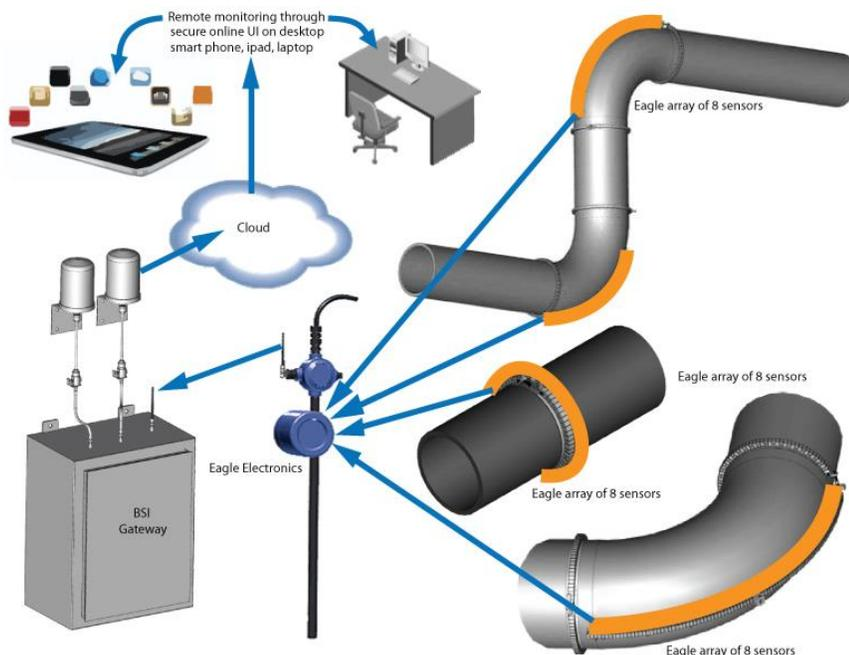
Figure 8. Mechanical integrity monitoring wireless network configuration.
