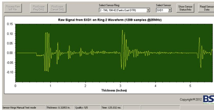
Figure 3. B-scan ultrasound echoes acquired from the pipe’s surface and remotely monitored and available to the user on-line.
