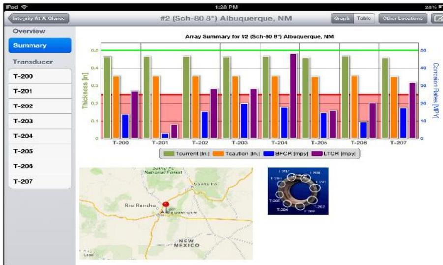
Figure 5. Summary of all arrays located on one pipe segment or pipeline. Pipe location coordinates and geo-location are provided.
